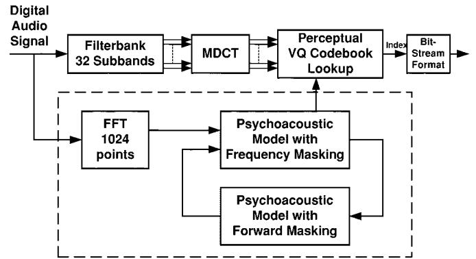
Fig. 10. Architecture of the proposed perceptual VQ-based audio coding system.
