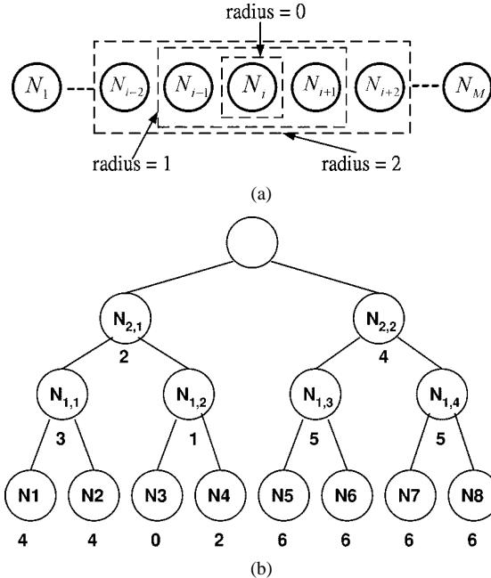
Fig. 7. (a) One-dimensional neuron structure in SOFM and (b) binary tree neuron structure in BT-SOFM.
