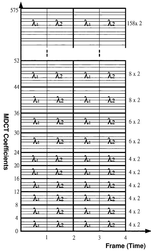
Fig. 11. Definition of critical band vectors used in the proposed audio coding scheme.
