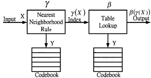
Fig. 6. Architecture of a vector quantization system.
