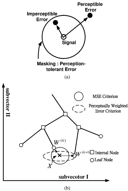
Fig. 12. (a) Concept of masking region in vector quantization and (b) perceptually weighted error criterion used in searching for the nearest codeword.
