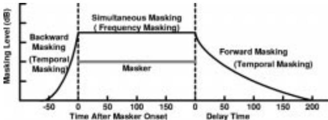
Fig. 1. Frequency and temporal masking effects.
