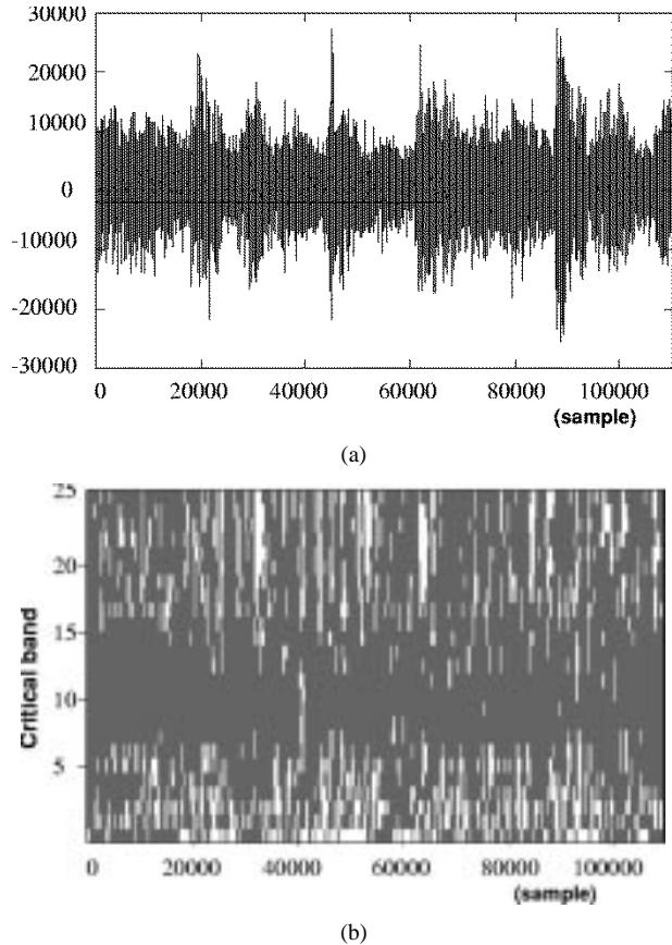
Fig. 5. (a) Piece of orchestra music and (b) the dominance pattern in the time-frequency space: simultaneous (frequency) masking effect (black) and forward masking effect (white).
