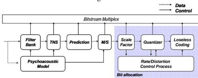
Figure 1: Block diagram of AAC encoder
