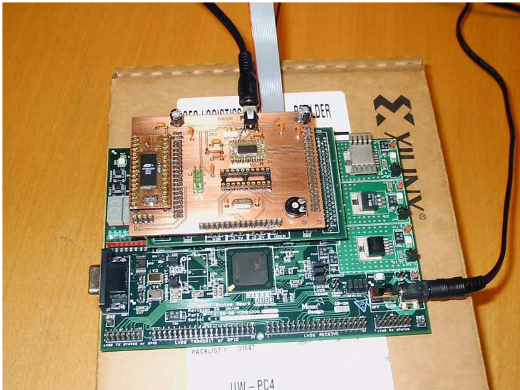
Fig. 8. Xilinx devel board, DAC board
