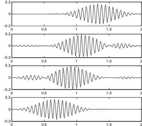
Figure 2. Some of the NMLBT synthesis functions when the combination matrix is switched on. Horizontal scale = block length.
