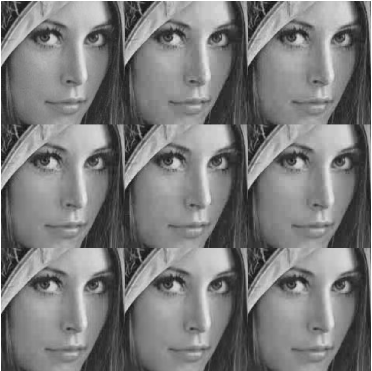
Figure 16. Coding examples for image “lena2” at 0.5 bits/pixel. Top row, left to right: original, JPEG encoding with DCT, and JPEG/LOT, PSNR (dB) = 32.0 and 32.3. Middle row: JPEG/LBT, JPEG/HLBT, and EZDCT with PSNR (dB) = 32.7, 32.4, and 32.9. Bottom row: EZ/LOT, EZ/LBT, and EZ/HLBT, with PSNR (dB) = 33.4, 34.0, and 33.5.
